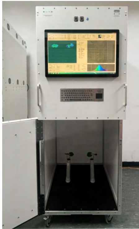
Figure 2. Image of the CropReporter with two plants placed inside the imaging chamber (source: Lazarevic B, 2023).
